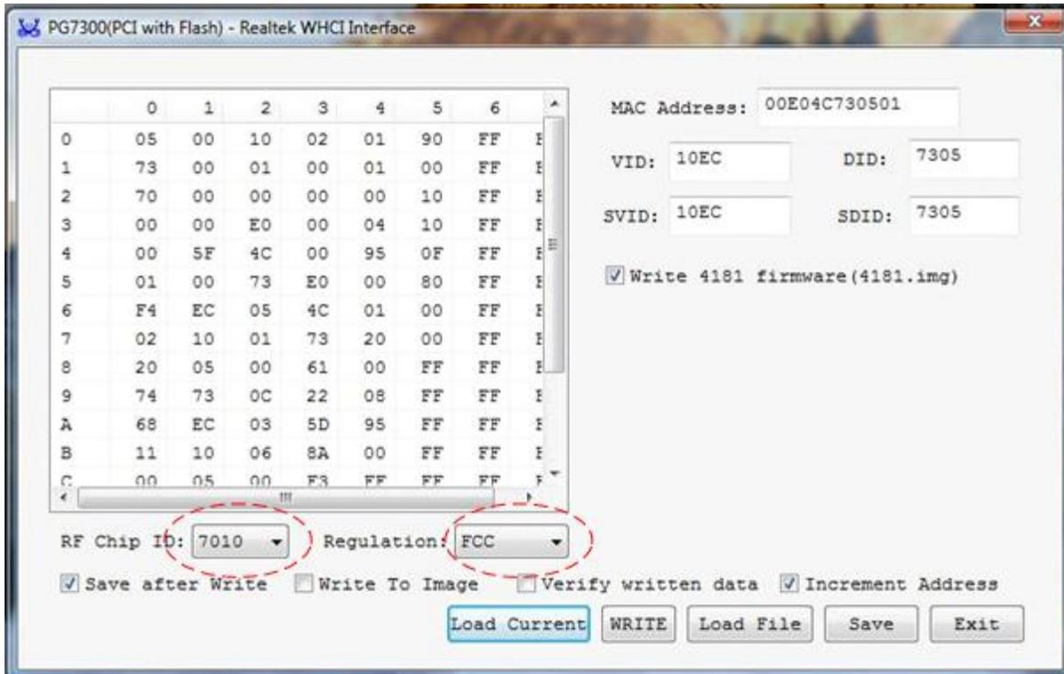
4. Check the module at your hand is RTU7010(BG1) or RTU7012(BG1&3). Also refer to your Realtek contact about the region support(FCC or TELEC) of that module. Then select the appropriate “Chip ID” and “Regulation”.
